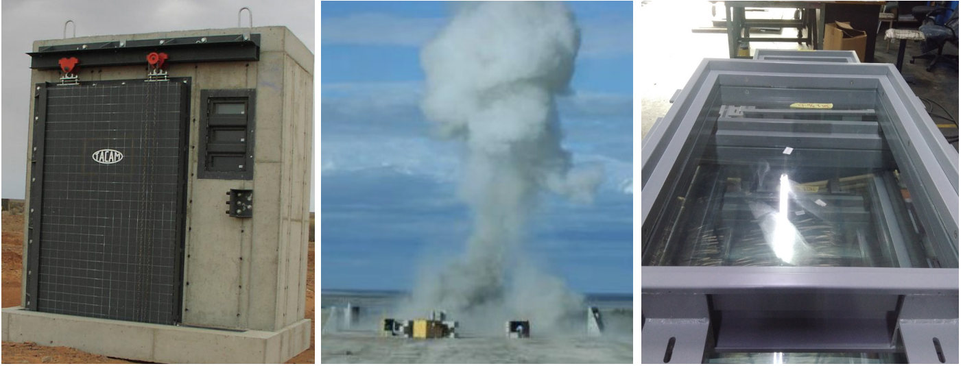
Sliding door and window in physical testing. Blast resistant windows are available too.
