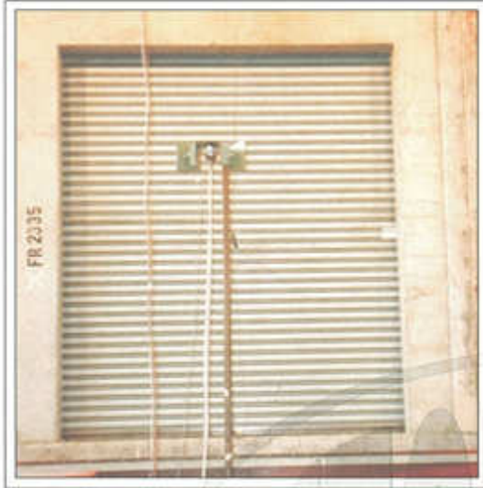
TACAM Shutter at START of 4 Hours Fire Test at SIRIM
