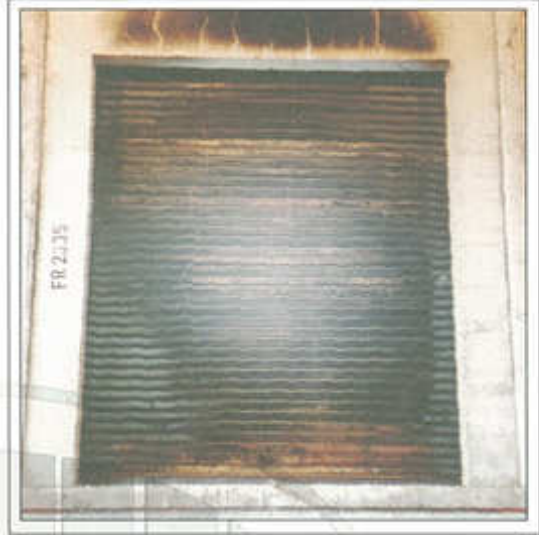
TACAM Shutter AFTER conclusion of 4 hours Fire Test. Fully intact; minimum distortion.
